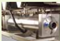
Cooler aluminium protective cladding
